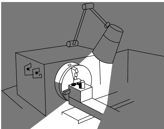
Figure 1.6 Local lighting on a centre lathe
